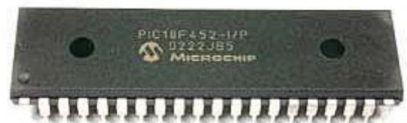
Figure 3. Photograph of PIC18F452 microcontroller
