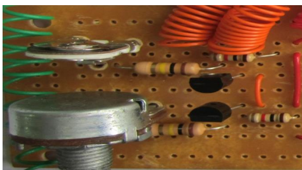
Figure 7. Photograph of water level sensor circuit
